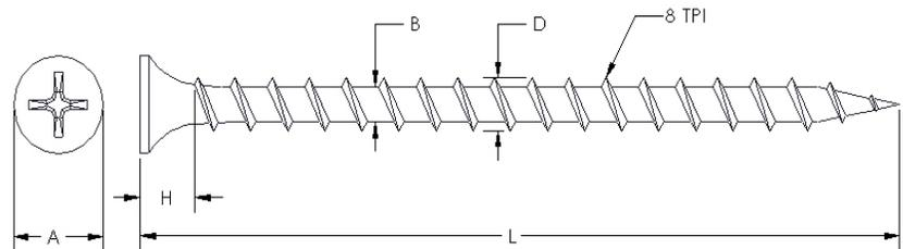
Fasteners comply with ASTM C1002 Type W
