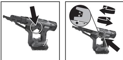
2. Adjust the countersink by turning the depth adjustment thumbwheel.
