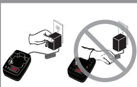
● To reduce risk of electric shock, unplug charger from outlet by wall mount unit. Do not unplug charger by pulling on cord.
