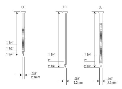
15 Degree Wire Welded or Plastic Carrier Coil
